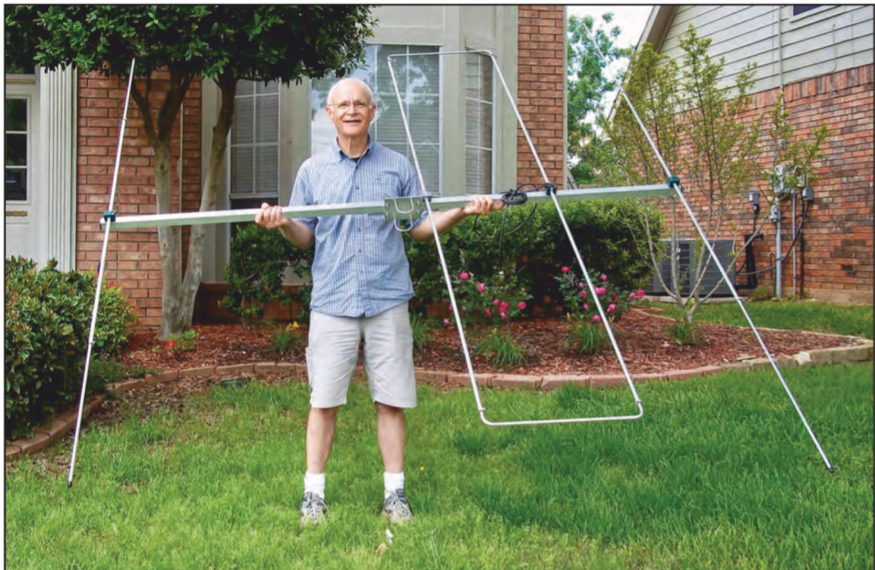
Photo A. Three-element LFA Yagi with K5ND. This antenna can fit in your backyard and works great six-meter DX.
