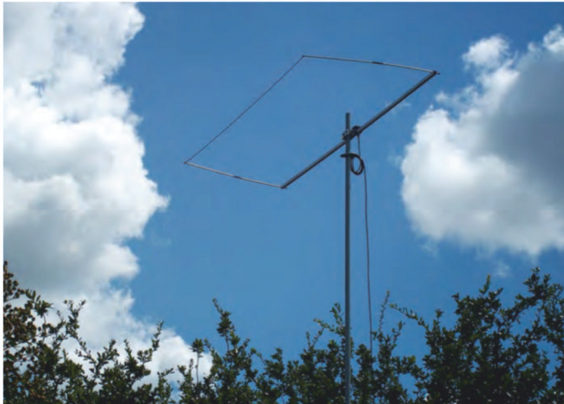
Photo B. Six-meter Stressed Moxon from Par Electronics. Compact at 84 x 31 inches and lightweight.
