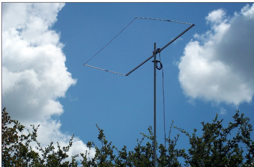
Six-meter stressed Moxon from PAR Electronics.
