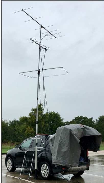
The K5ND/r push-up mast in the rain during the ARRL 2018 September VHF Contest. Note the stand-up position in the back along with the tarp to provide some protection from the rain.
