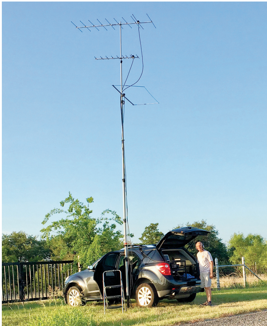
Evolution of the K5ND roving setup, with an improved Fiberglass mast and stand-up operating position.
