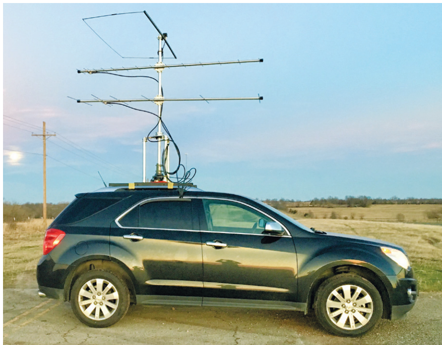
A rooftop rotator is added for immediate operation.
