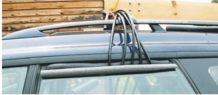
Figure 2 — Pool noodles or foam blocks get your feed lines into the vehicle with some weather protection. Slit the foam to seat on the glass or frame and raise the window until the feed lines are securely held. [James Duffey, KK6MC, photo]
