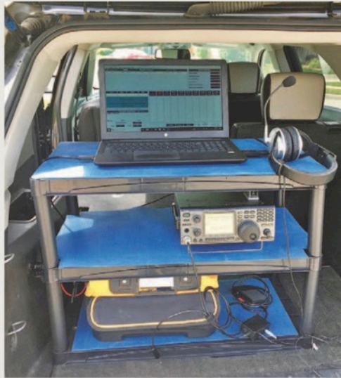
Figure A — The rover's radio equipment is set up on a self-contained shelving unit with the shelves adjusted to fit the equipment. [Jim Wilson, K5ND, photo]
