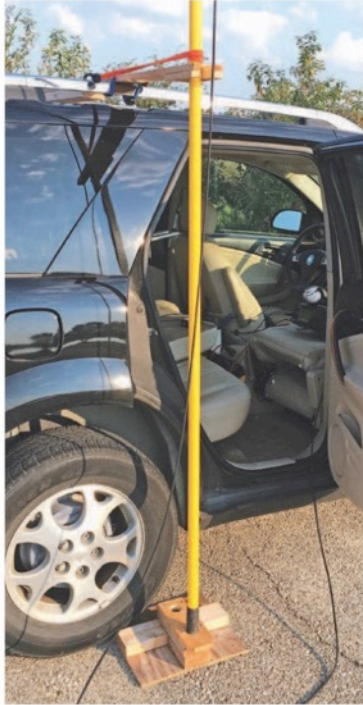
Figure 1 — Jim's, K5ND, drive-on base secures the bottom of his painter's pole, and he stabilizes the mast with an attachment to a roof rack. [Jim Wilson, K5ND, photo]
