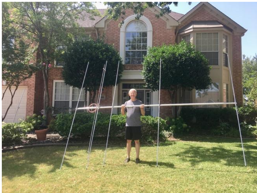
Figure 23 - Directive Systems 5-element Yagi
