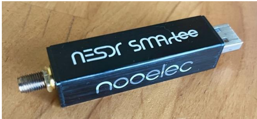
Figure 66 - RTL-SDR Dongle Receiver
