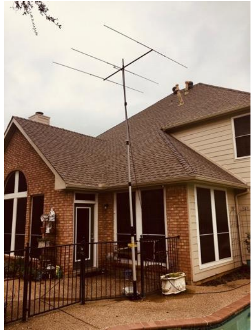
Figure 22 - M2 3-element Yagi
