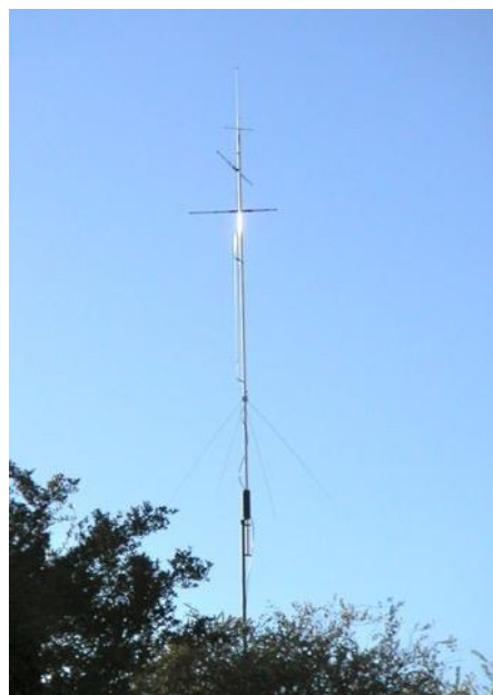
Figure 19 - MA6V vertical dipole for 20-6 meters.
