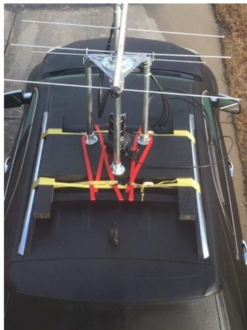
Figure 63 - Rooftop mounting system
