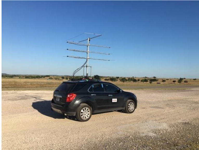
Figure 32 - K5ND/R with 50, 144, 220, 432 antennas
