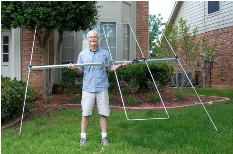
Figure 22 - Innovantennas 3-element Yagi
