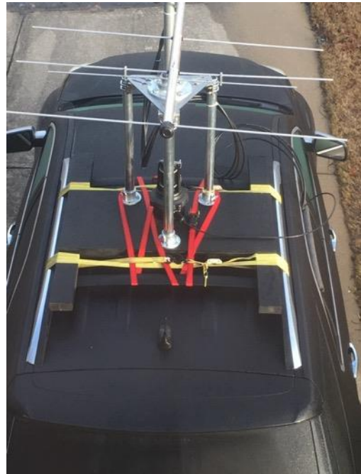
Figure 52 - Rooftop mounting system
