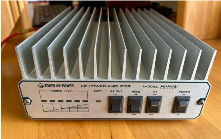
Figure 16 - Tokyo Hy-Power 6 meter amplifier 160 watts
