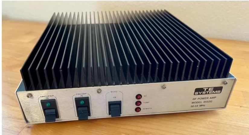
Figure 14 - TE Systems 375 Watt Six Meter Amplifier
