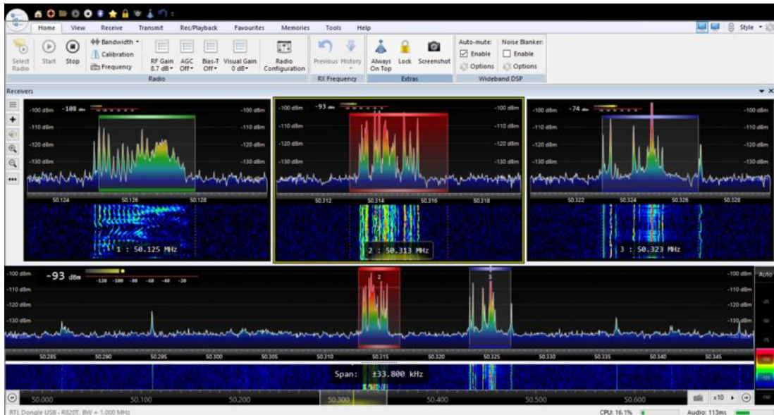
Figure 59 - Receivers covering 50.125 SSB, 50.313 FT8, and 50.323 FT8 to Europe
